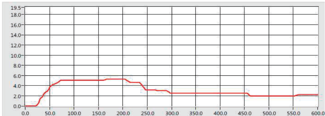
Graph No. 1 - Flame Spread Distance Versus Time
