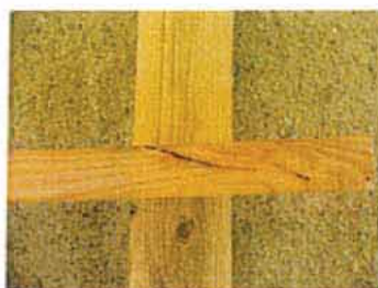
KY1, Chip, (Thickness:21mm, Width:24mm)
