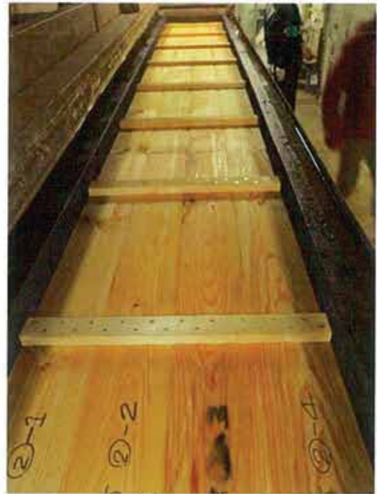
After testing (unexposed side,far side of burner)
