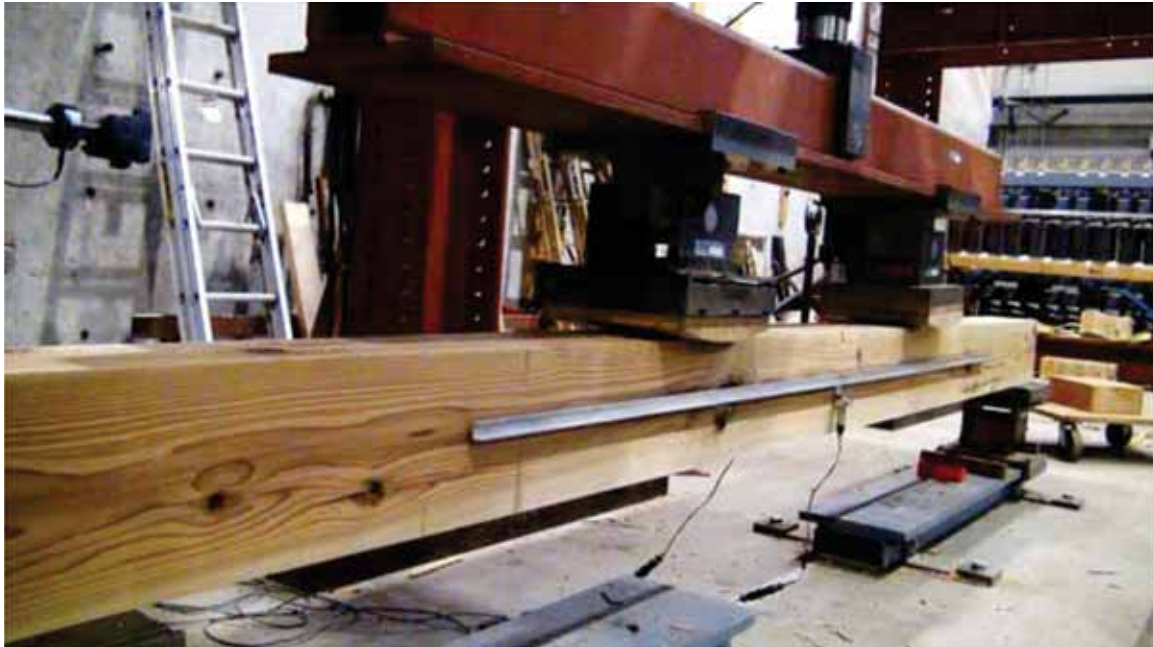
Figure 1 Static bending test setup
